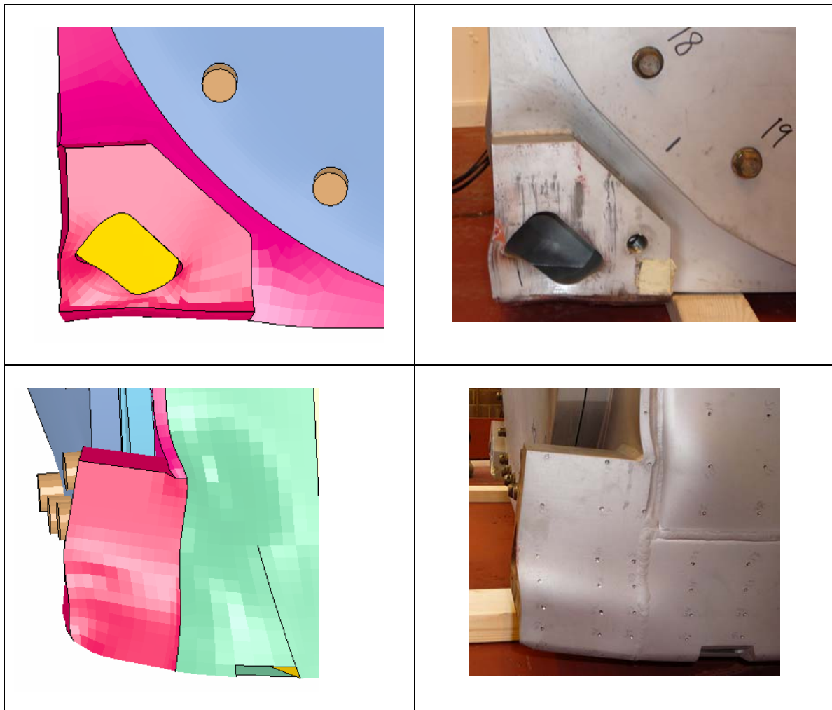
Figure 2: Comparison of Knock-back Between Finite Element Prediction and Test.
