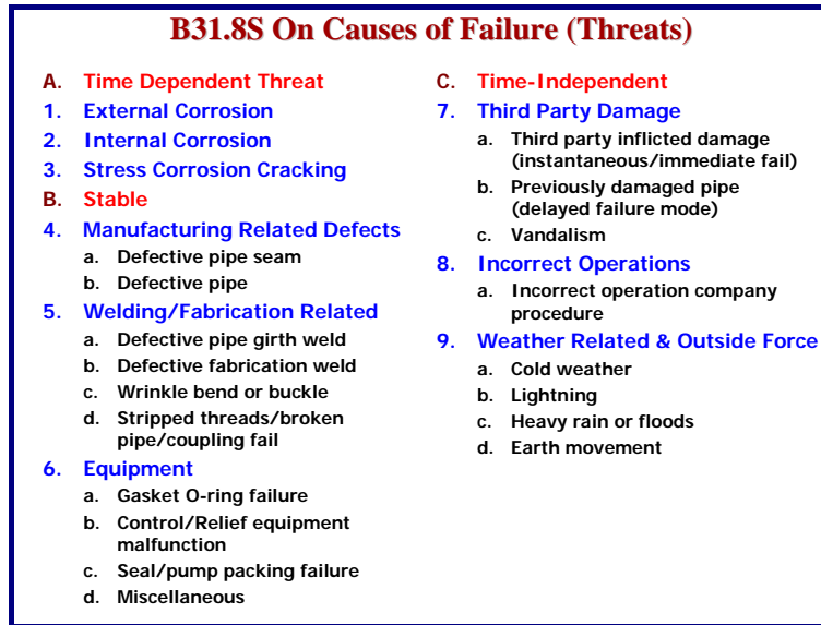
Figure -3 Pipeline Failure Threats
